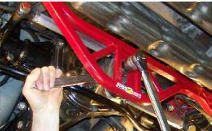
Propeller bolt and nut (3/4 x 3.0 x 10)
