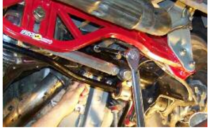
Drivers side axle clamps bolts and nuts (1/2 x 2.25)
