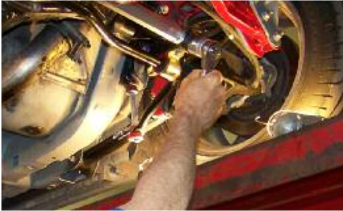
Drivers side watts bars bolt (3/4 x 3.5 x 16)
