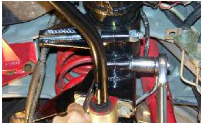
Drivers side axle clamps bolts and nuts (1/2 x 2.25)
