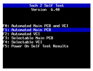
FIGURE 6-9. Automated Main PCB Test Selected on Tech 2 Self Test Main Menu
