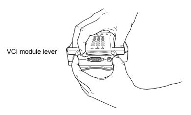
FIGURE 3-11. VCI Module Removal
