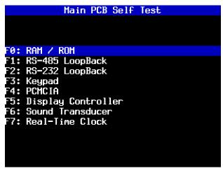
FIGURE 6-12. Selectable Main PCB Self Test Screen
