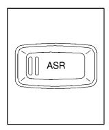
To turn the system off, press the ASR button located on the instrument panel.
